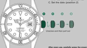
back down against the case to guarantee the waterproofness. Return the crown to position 1 and apply light pressure on it while screwing it down clockwise against the case. The crown should never be unscrewed underwater.
